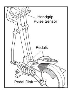
either direction. It is recommended that you move the pedal disks in the direction shown by the arrow; however, for variety, you may turn the pedal disks in the opposite direction.
